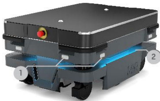
Figure 5.6 Light indicators on MiR250 Shelf Carrier
