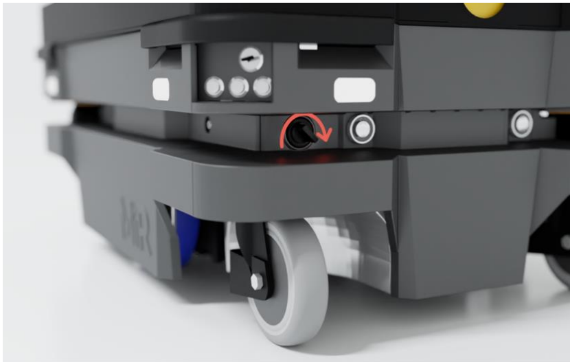
Figure 5.5 Turn the Manual brake release switch clockwise to release the brakes
