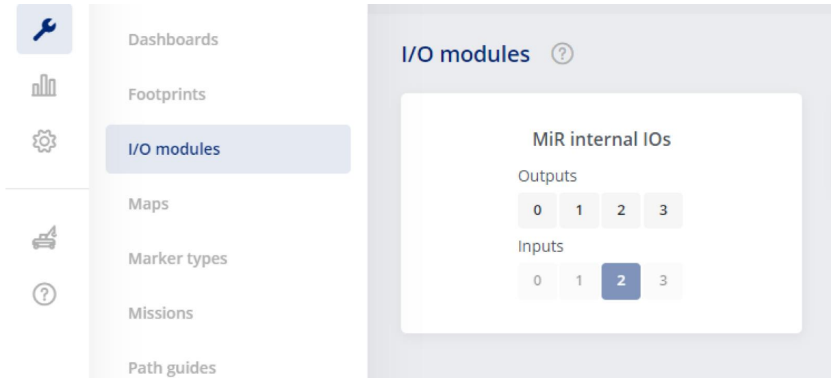
Figure 17.4 Example of input 2 registered as active by the robot
