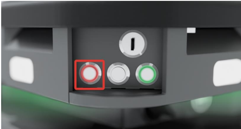
Figure 5.4 The Manual stop button is the left-most button on the control panel
